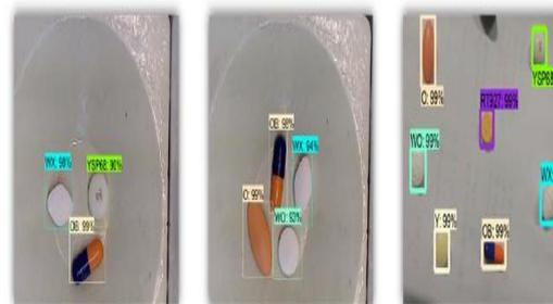
Fig. 7. Photographs captured during the actual drug recognition process and the recognition results generated by the proposed intelligent medicine device.
