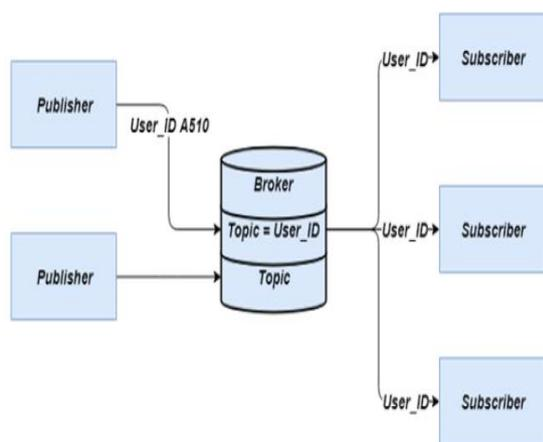
Fig. 2. The MQTT architecture.
